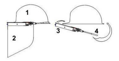
1 Helmet 2 Face shield 3 Visor carrier 4 Tension spring
